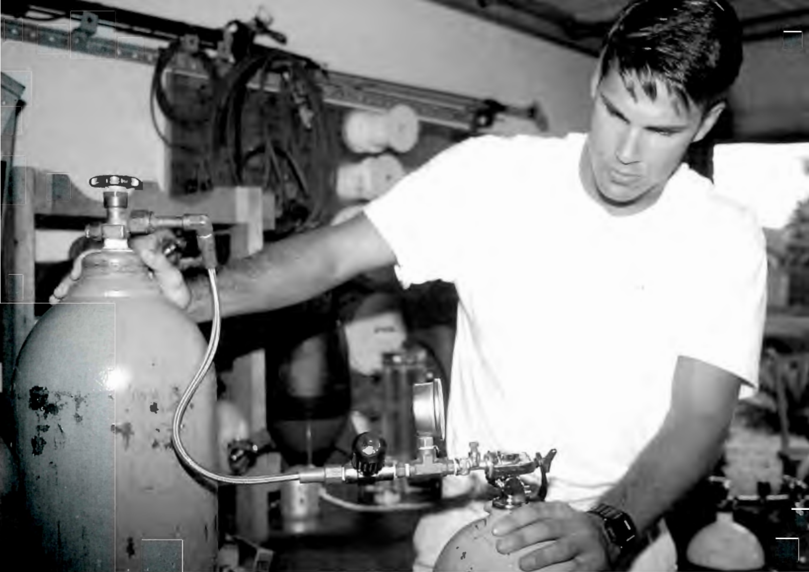
Partial pressure filling is accomplished by partially filling a scuba cylinder with one or more gases by connecting it to larger cylinders via a fill whip and opening the valves of both cylinders. The gas flows from the cylinder with the greatest pressure, the supply cylinder, to the cylinder being filled, the scuba cylinder.
