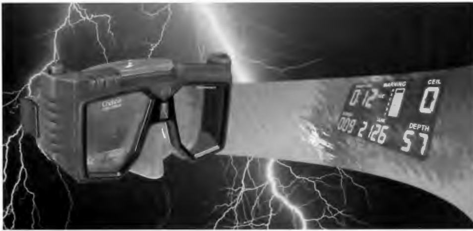
Spectacle is a futuristic mask that projects a virtual image of the Nemesis computer data into the divers field of vision. From the divers perspective, it appears that the ghost-like image is suspended in the water in the lower right hand side of the divers field of vision.
